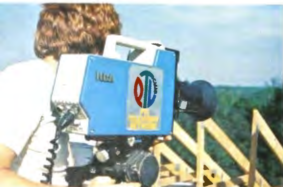
Camera complement at PTL includes the TK-76 as well as TK-46, TKP-45 and TK-44 cameras.
