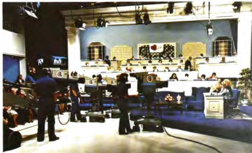
Four TK-46 cameras are used to cover the PTL Club production. The L-shaped studio has about 9,000 square feet of floor space and includes a 208 seat theatre.
