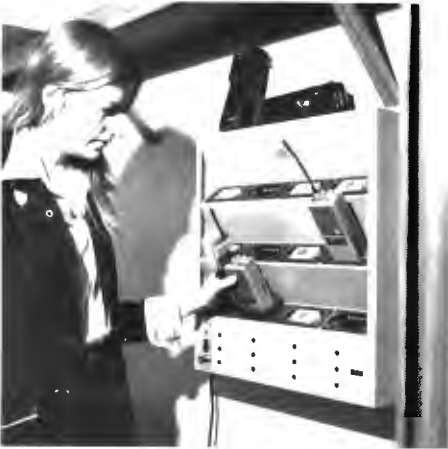
In addition to the VEETAC mobile units in the vehicles, TV-39 uses RCA TACTEC hand-held portable radios for use outside of the mobile units. When not in use, these are stored in the charging unit shown.
