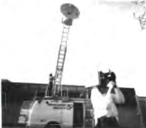
One ENG van is equipped with a Van Ladder to raise the microwave dish for best line-of-sight transmission.
